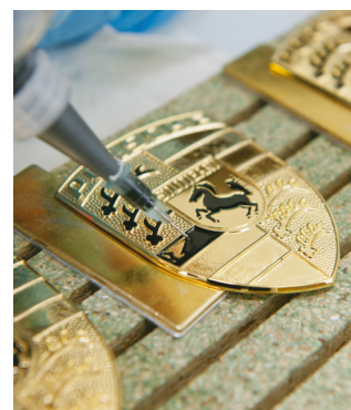
Applying the enamel by hand
